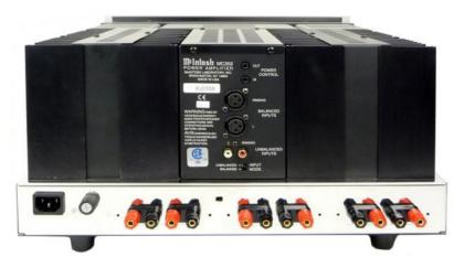
BACK PANEL: POWER CONTROL jacks: OUT and IN. BALANCED Right/MONO and Left INPUTS. UNBALANCED Left and Right/MONO INPUTS. INPUT MODE switch: BALANCED or UNBALANCED.  $\checkmark$  Power cord receptacle. FUSE. Gold plated RIGHT channel OUTPUT terminals for 4, or 8 Ω speakers. OUTPUT MODE switch: MONO/PARALLEL or STEREO. RIGHT and LEFT gold plated speaker OUTPUT terminals for 2 Ω. Gold plated LEFT channel OUTPUT terminals for 4, or 8 Ω speakers.
