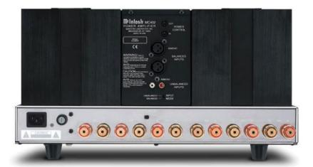
BACK PANEL: POWER CONTROL jacks: OUT and IN. BALANCED Right/MONO and Left INPUTS. UNBALANCED Left and Right/MONO INPUTS. INPUT MODE: UNBALANCED or BALANCED.  $\checkmark$  Polished stainless steel chassis. Power cord receptacle. FUSE. RIGHT channel OUTPUT binding posts for 2  $\Omega$ , 4  $\Omega$  or 8  $\Omega$  speakers. LEFT channel OUTPUT binding posts for 2  $\Omega$ , 4  $\Omega$  or 8  $\Omega$  speakers.
