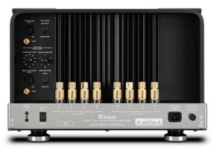
BACK PANEL: Polished stainless steel/black chassis. VACUUM TUBE INPUT: BALanced and UNBALanced. ☆ INPUT MODE selector switch: BALANCED or UNBALANCED. ☆ CROSSOVER (MONO MODE) control: CROSSOVER POINT (HZ): 100, 130, 180, 250, 300, 400, 550, 800, 1K. VACUUM TUBE LEVEL control: (DB) -6, -3, 0, +1.2, +3. ☆ MONO/SOLID STATE INPUT: BALanced and UNBALanced. AMPLIFIER MODE switch: MONO or SEPARATE. ☆ VACUUM TUBE OUTPUTS:
