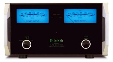
**FRONT PANEL:** LED/fiber-optic illuminated green/gold nomenclature. Left illuminated **POWER OUTPUT** meter (linear WATTS or DECIBELS). LEFT and RIGHT POWER GUARD LEDS. Right illuminated POWER OUTPUT meter (linear WATTS or DECIBELS). Standby power on indicator. METER mode switch: LIGHTS OFF, WATTS or HOLD. POWER switch: OFF, REMOTE or ON. Handles.
