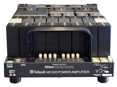
**BACK PANEL:** Power cord receptacle. **CIRCUIT BREAKER. POWER CONTROL** jacks: **IN** and **OUT**. **LEFT** and **RIGHT** gold plated speaker **OUTPUT** terminals. **LEFT** and **RIGHT BALANCED** audio **INPUT**. **LEFT** and **RIGHT UNBALANCED** audio **INPUT**. **MODE** switch: **STEREO** or **BRIDGED**. Early units had black-painted chassis - later units had stainless steel chassis.
