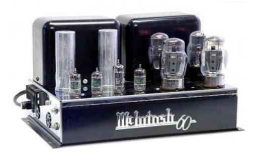
CONTROLS & CONNECTORS: Chrome/black chassis. Power cord. Speaker OUTPUT barrier strip for 4, 8 and 16 ohms as well as 0.5V INPUT. 0.5V INPUT. GAIN control. FUSE. 3 AMP AC OUTLET. Octal OUTPUT socket powers McIntosh C 8, C 4, C 104, or C 108 preamps. Octal socket PRE-AMP. INPUT. HUM ADJUSTMENT.
