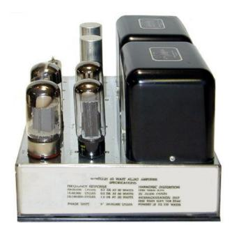
SPECIFICATIONS: 60w. Response: 20-30kHz (+0.1-0.1dB). Distortion: 0.5%. Noise & Hum: - 90dB. Output Impedance: 4, 8, 16, and 600 ohms. 600 ohm balanced to ground. 4, 8 and 16 ohms isolated from ground. Damping Factor: 12 for 4, 8 and 16 ohms. Input Impedance: 500k. Input Sensitivity: 0.5V. Unity Coupled.
