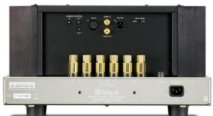
**BACK PANEL:** POWER CONTROL jacks: IN, OUT 1 and 2. BALanced INput. INput/OUTput. BALanced OUTput. INPUT MODE switch: UNBALanced or BALanced. Polished stainless steel chassis. Gold plated output terminals for 8  $\Omega$ , 4  $\Omega$ , or 2  $\Omega$ speakers. **FUSE**. Power cord receptacle.
