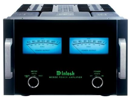
FRONT PANEL: Glass with illuminated green/gold nomenclature. Illuminated left and right POWER OUTPUT meters (linear WATTS or DECIBELS). Left and right POWER GUARD lights.
