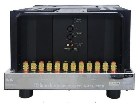
**BACK PANEL:** POWER CONTROL jacks: OUT and IN. LEFT and RIGHT BALANCED INPUTS. LEFT and RIGHT UNBALANCED INPUTS. INPUT MODE switch: BALANCED or UNBALANCED.  $\checkmark$  Polished stainless steel chassis. CIRCUIT BREAKER. Gold plated RIGHT channel OUTPUT terminals for 2, 4, or 8  $\Omega$  speakers. Gold plated LEFT channel OUTPUT terminals for 2, 4, or 8  $\Omega$  speakers. Power cord receptacle.
