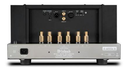
**BACK PANEL:** POWER CONTROL jacks: IN, OUT 1 and 2. BALanced OUTput. UNBALanced: INput/OUTput. BALanced INput. AUTO OFF: ENabled or DISabled. INPUT MODE switch: UNBALanced or BALanced.  $\checkmark$  Polished stainless steel chassis. FUSE. Gold plated OUTPUT terminals for 8  $\Omega$ , 4  $\Omega$ , or 2  $\Omega$  speakers.  $\checkmark$  Power cord receptacle.
