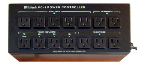
**TOP PANEL:** Black chassis. 5 switched AUDIO UNITS AC outlets (with indicator light). 2 switched VIDEO UNITS AC outlets (with indicator light). ★ 4 switched POWER AMPLIFIERS AC outlets: MAIN, 2, 3, and 4 (with individual indicator lights). 3 UNSWITCHED AC outlets (with indicator light).
