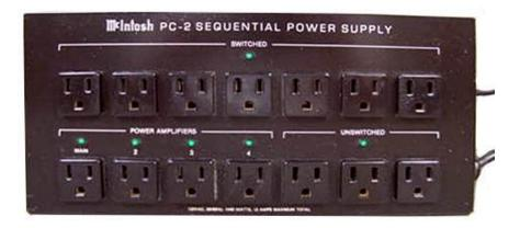
**TOP PANEL:** Black chassis. 7 switched AUDIO UNITS AC outlets (with indicator light). 4 sequentially switched **POWER AMPLIFIERS** AC outlets: MAIN, 2, 3, and 4 (with individual indicator lights). 3 UNSWITCHED AC outlets. LED AC power indicator.
