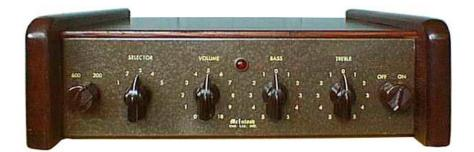
FRONT PANEL: Brown hammer tone finish. Turnover: 600 or 300Hz at 6dB/octave. Input SELECTOR: 1 (GE cartridge), 2 (Pickering cartridge), 3 (crystal cartridge), 4 (tuner), 5 (microphone). VOLUME: 0 to 10. BASS boost: 0 to 5, cut: 0 to 5. Power indicator light. TREBLE boost: 0 to 5, cut: 0 to 5. Power switch: OFF or ON. Mahogany finish wood case.
