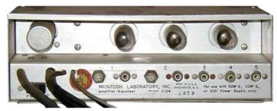
**BACK PANEL:** Power cord. Output to power amp. Inputs: 1 (tuner)(with trim), 2 (low level magnetic pickup) (with trim), 3 (high level magnetic pickup), 4 (crystal pickup) and 5 (low level microphone).
