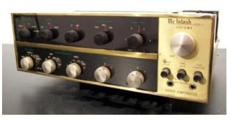
C 20 (EARLY) "Spotting features": 1. Front panel is plastic with brass bar separating the upper and lower panel. 2. Top panel covers the front panel lights. 3. Volume control is exposed. 4. Transformer is un-potted. 5. Thin, fixed end caps.
