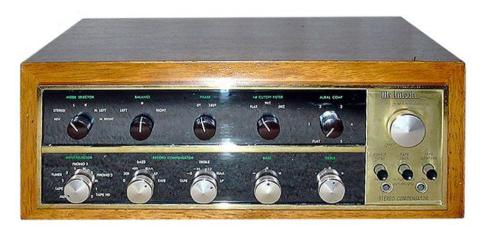
FRONT PANEL: Plastic panel with brass trim. Mode Selector: Reverse, Stereo, L, R, M
