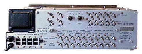
BACK PANEL: OUTPUTS: L&R MAIN, L&R TAPE. L&R LOW FREQUENCY TRIM controls. HIGH LEVEL INPUTS: TAPE COMPARE, AUX, TAPE, TUNER 1, TUNER 2.
