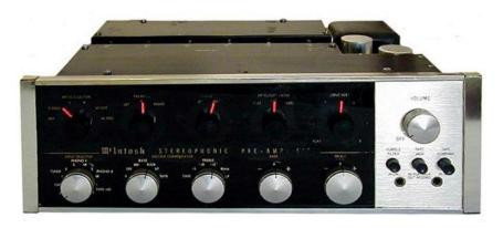
FRONT PANEL: Glass panel with illuminated teal/gold nomenclature and gold anodized aluminum trim. Mode Selector: Reverse, Stereo, L, R, M Left, M RIGHT. BALANCE: Left, 0, or RIGHT. PHASE: 0 or 180. HF CUTOFF FILTER: FLAT, 9KC or 5KC. LOUDNESS: FLAT, 1 to 5. VOLUME with on-OFF switch.
