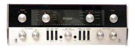
FRONT PANEL: Glass with gold nomenclature and gold anodized panel. BALANCE: LEFT to RIGHT. INPUT selector (with indicator lights): AUX, TAPE, TUNER 2, TUNER 1, PHONO 1, PHONO 2, MIC and TAPE HD. MODE SELECTOR (with indicator lights): L TO L+R, R TO L+R, STEREO REVERSE, STEREO, MONO (L+R), L+R TO L and L+R TO R. VOLUME.
