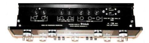
**TOP PANEL:** TAPE EQUALIZATION: L and R with NAB mark. LOW FREQUENCY TRIM: L and R. OUTPUT LEVEL: Left, L+R and Right. PHASE switch: REVERSE (180°) or NORMAL (0°). PILOT LAMP INTENSITY: DIM or BRIGHT.
