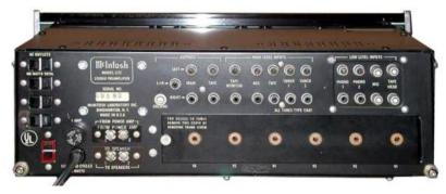
BACK PANEL: AC OUTLETS: 4 switched, 1 unswitched. FUSE. Power cord. Screw terminals: left speaker FROM POWER AMP and TO SPEAKER (for phase switch). ✓ GROUND binding post. OUTPUTS: L+R, MAIN, TAPE. HIGH LEVEL INPUTS: TAPE MONITOR, AUX, TAPE, TUNER 1, TUNER 2. LOW LEVEL INPUTS: PHONO 1, PHONO 2, MIC, TAPE HEAD.
