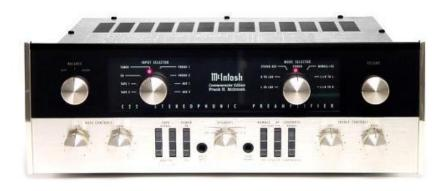
FRONT PANEL: Glass with illuminated teal/gold nomenclature and gold anodized aluminum panel. BALANCE: LEFT to RIGHT. INPUT SELECTOR (with indicator lights): TAPE 2, TAPE 1, CD, TUNER, PHONO 1, PHONO 2, AUX 1, AUX 2. MODE SELECTOR (with indicator lights): L TO L+R, R TO L+R, STEREO REV, STEREO, MONO (L+R), L+R TO L and L+R TO R. VOLUME.
