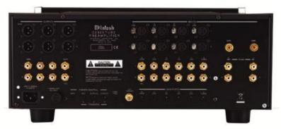
BACK PANEL: Left and Right balanced OUTPUTS: MAIN, 2, and 1. Left and Right balanced INPUTS: 7-CDR, 6-CD, 5-DA and 4-DVD. 2 Ground binding posts.
