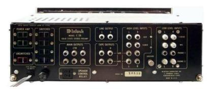
BACK PANEL: AC outlets: 2 POWER AMP (switched at top panel), 1 UNSWITCHED, 4 SWITCHED (at front panel). Power cord. FUSE. MAIN OUTPUTS (2 pair): L, Center, R. SPEAKER CONTROL RELAY socket. Left and Right LINE OUTPUT. TAPE 1 and TAPE 2 Left and Right OUTPUTS. HIGH LEVEL INPUTS: AUX, TUNER, TAPE 1, TAPE 2. GROUND binding post. LOW LEVEL INPUTS: Tape HEAD, MIC, PHONO 1 and PHONO 2. Panloc mounting.
