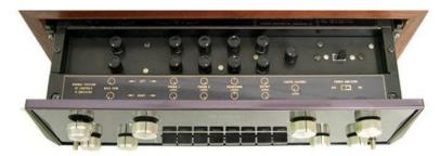
**TOP PANEL:** LEFT and RIGHT BASS trim. LEFT and RIGHT PHONO 1 and PHONO 2 LEVEL controls. LEFT and RIGHT HEADPHONES LEVEL controls. LEFT and RIGHT OUTPUT LEVEL controls. CENTER CHANNEL LEVEL control. POWER AMPLIFIER Switch: OFF or ON.
