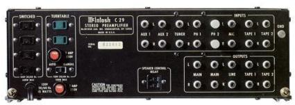
BACK PANEL: 4 SWITCHED AC outlets. 2 UNSWITCHED AC outlets (TURNTABLE auto-on).
