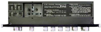
**TOP PANEL:** MONITOR AMPLIFIER CONTROLS: LEFT GAIN, INPUT switch: RECORD or <u>LISTEN</u> and RIGHT GAIN. EXPANDER controls: LEVEL MATCH, SPEED: FAST, NORM and SLOW.
