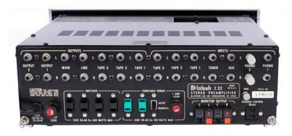
BACK PANEL: OUTPUTS: 2, 1, MAIN, LINE, TAPE 3, TAPE 2, TAPE 1. INPUTS: TAPE 3, TAPE 2, TAPE 1, TUNER, AUX, PHONO 2, PHONO 1.
