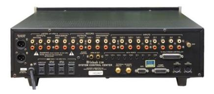
BACK PANEL: Left and Right BALANCED OUTPUTS. LISTEN: OUTPUTS: SWITCHED: 2 and 1, MAIN and PROCESSOR: FROM and TO. RECORD: OUTPUTS: TAPE 3, TAPE 2, TAPE 1 and PROCESSOR: FROM and TO. AUDIO INPUTS: VIDEO, TAPE 3, TAPE 2, TAPE 1, TUNER, CD 2, CD 1, AUX, PH. Ground binding post.
