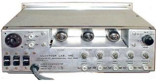
**REAR PANEL:** Octal power and audio output socket. **OUTPUTS**: **TAPE** and **MAIN**. Tube cover. **PHONO 2 LOAD** switch: **6.8K** to **52K**.
