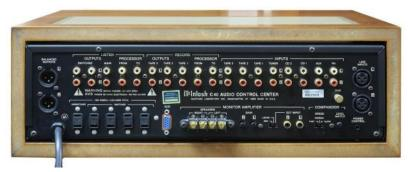
BACK PANEL: Left and Right BALANCED OUTPUTS. LISTEN OUTPUTS: SWITCHED: 1 and 2, MAIN, PROCESSOR: FROM and TO. RECORD OUTPUTS: TAPE 3, TAPE 2, TAPE 1, PROCESSOR: FROM and TO. Audio INPUTS: TAPE 3, TAPE 2, TAPE 1, TUNER, CD 2, CD 1, AUX, PH. GROUND binding post. Left and Right BALANCED INPUTS.
