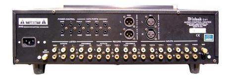
BACK PANEL: POWER CONTROL jacks: MAIN, ACCESSORY, amplifier 1 and amplifier 2. DATA PORTS: PH/AUX, VIDEO, TUNER, T3/DVD, CD 2, CD 1, TAPE 1, TAPE 2. Left and Right BALANCED MAIN OUTPUTS. Left and Right BALANCED CD1 INPUTS.
