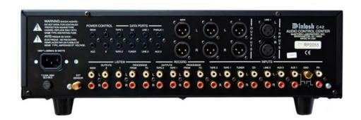
BACK PANEL: POWER CONTROL jacks: MAIN, ACCESSORY, amplifier 1 and amplifier 2. DATA PORTS: TAPE 1, TAPE 2, CD, TUNER, LINE 1, LINE 2, PH/AUX 1, AUX 2. Left and Right BALANCED OUTPUTS: MAIN, 2 and 1. Left and Right BALANCED LINE 1 INPUTS.
