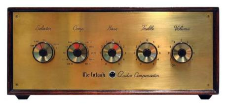
FRONT PANEL: Brass finish. SELECTOR: TAPE, TUNER, MIC, PHONO 1, PHONO 2. COMP: 629.16, 629.11, 800.16, 800.10. BASS boost: 0 to 5, cut: 0 to 5. TREBLE boost: 0 to 5, cut: 0 to 5. VOLUME: 1 to 10 with on-OFF switch.
