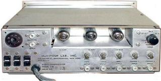
**REAR PANEL:** Octal power and audio output socket. **OUTPUTS: TAPE** and **MAIN**. Tube cover. **PHONO 2 LOAD** switch: **6.8K** to **52K**.
