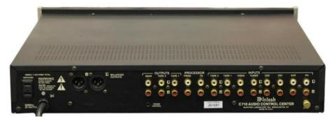
BACK PANEL: SWITCHED AC outlet. Right and Left BALANCED OUTPUTS. OUTPUTS: MAIN, TAPE 2, TAPE 1. PROCESSOR: FROM and TO. INPUTS: TAPE 2, TAPE 1, VIDEO, TUNER, CD2, CD1, AUX, PH.
