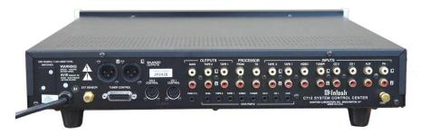
BACK PANEL: SWITCHED AC outlet. Right and Left BALANCED OUTPUTS. OUTPUTS: MAIN, TAPE 2, TAPE 1. PROCESSOR: FROM and TO. INPUTS: TAPE 2, TAPE 1, VIDEO, TUNER, CD2, CD1, AUX, PH.
