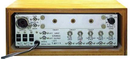
BACK PANEL: Octal power and audio output socket. OUTPUTS: TAPE and MAIN. Tube cover. PHONO 2 LOAD control: F.M., 2K, 7K, 36K, 47K, 52K.
