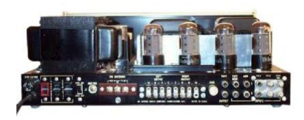
BACK PANEL: FUSE. Power cord. AC OUTLETS: 1 unswitched, 2 switched. Speaker switch: ON Or OFF. MUTING adjustment. Screw terminals for FM ANTENNA: 300  $\Omega$  and 75  $\Omega$ . LEFT and RIGHT OUTPUT barrier strip terminals for 4  $\Omega$ , 8  $\Omega$ , and 16  $\Omega$  speakers. Ground terminal. TAPE OUTPUT. INPUTS: TAPE MON, AUX, PH 1, PH 2, TAPE HEAD.
