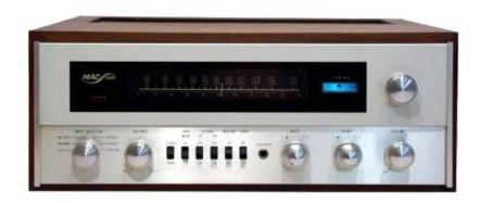
FRONT PANEL: Anodized aluminum panel. Illuminated tuning dial. TUNING meter. Tuning control.
