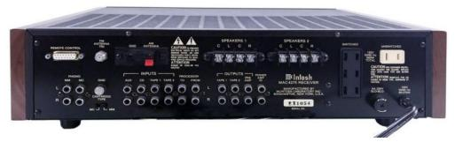
BACK PANEL: 15 pin REMOTE CONTROL receptacle. 75 Ω FM ANTENNA coax input. Push terminals: Ground and AM ANTENNA. Left and Right output screw terminals: SPEAKERS 1 and 2. AC outlets: 3 SWITCHED, 1 UNSWITCHED.
