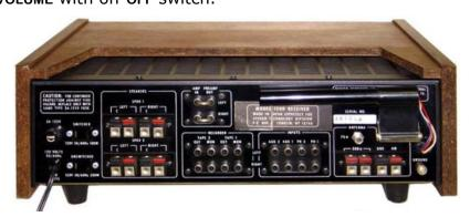
BACK PANEL: FUSE. Power cord. AC outlets: 1 SWITCHED, 1 UNSWITCHED.  $\checkmark$  Output SPEAKERS push terminals: LEFT and RIGHT SPEAKER 1 and 2.  $\checkmark$  LEFT and RIGHT jumpers: AMP IN and PREAMP OUT.  $\checkmark$  RECORDER: TAPE 2 OUT and MON, TAPE 1 OUT and MON. INPUTS: AUX 2, AUX 1, PH 2, PH 1. ANTENNA: 75  $\Omega$  FM ANTENNA coax input. Push terminals for 300  $\Omega$  FM antenna, GND and AM. Built-in ferrite AM loopstick. GROUND screw terminal.
