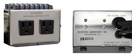
**FRONT PANEL:** Chrome and black chassis. Terminal strips: Input **FROM POWER AMPLIFIERS**: LEFT, CENTER and RIGHT. Output TO REMOTE SPEAKERS: LEFT, CENTER and RIGHT. Output TO MAIN SPEAKERS: LEFT, CENTER and RIGHT.
