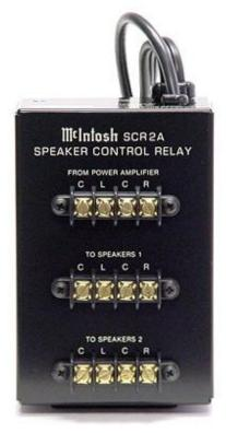
**FRONT PANEL:** Black chassis. Terminal strips: Input **FROM POWER AMPLIFIER**: LEFT and RIGHT. **CONTEXT OF CONTEXT OF SPEAKERS 1: LEFT** and RIGHT. **CONTEXT OF SPEAKERS 2: LEFT** and RIGHT.
