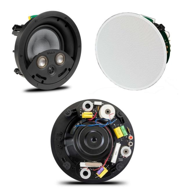
**DRIVERS:** 3-way system: one 8" woven glass fiber cone woofer; two 2" inverted titanium dome midrange and one 3/4" titanium dome tweeter.
