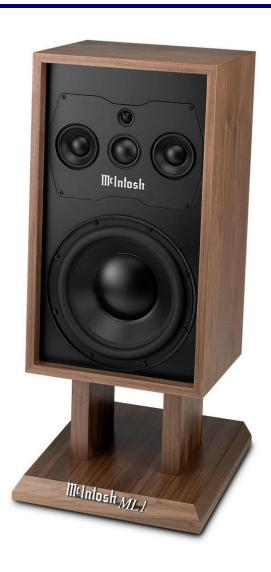
**DRIVERS:** 4-way system: one 12" LD/HP Woofer in a sealed enclosure, two 4" lower midrange drivers in a sealed enclosure, one 2" soft dome upper midrange and one 3/4" Titanium dome tweeter.
