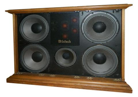
**DRIVERS:** 5-way system: with four 12" woofers, one 8" lower-mid, two 1-1/2" soft dome mid-mids, two 1-1/2" soft dome upper-mid, two 2-1/4" Peerless and one ½" super-radiator tweeters.
