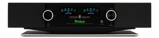
FRONT PANEL: Grille with black knit cloth. Glass with LED/fiber-optic illuminated green nomenclature. NETwork status indicator. Multi-function control: Select sources: BLUETOOTH, PHONO, HDMI, AUX, OPT / Adjust lighting / BlueTooth. Left illuminated digital OUTPUT LEVEL meter (dB). Right illuminated LED digital OUTPUT LEVEL meter (dB). Multi-function control: VOLUME with Minimum and Maximum volume indicators / POWER/MUTE / BASS ADJUSTMENT.
