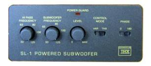
**FRONT PANEL:** Power switch with indicator lights: off or on/standby. High pass frequency control: 50 to 125Hz with labels at 50, 63, 80, 100 and 125Hz. Subwoofer frequency control: 50 to 125Hz with labels at 50, 63, 80, 100 and 125Hz. Level control: 0 to max. Control mode switch: variable or THX. Phase switch: 0 or 180.
