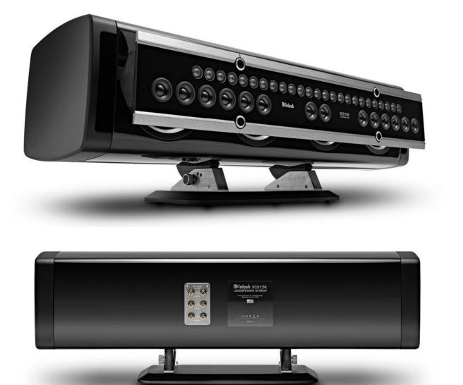
**DRIVERS:** 3-way system: Four 8" 8-Ohm long-throw carbon fiber sandwich cone Woofers, cascaded in pairs for woofer and MR bands. Fourteen 2.5" 4-Ohm aluminum dome Midranges. Twenty-five 3/4" 4-Ohm aluminum dome Tweeters.
