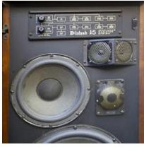
**DRIVERS:** 4-way system: one 12" woofer, one 8" lower mid, one 1-1/2" dome upper mid and two 5/8" angled Peerless tweeters.
