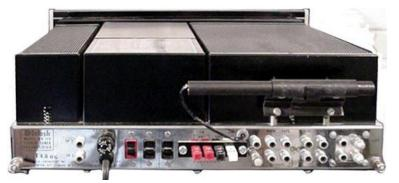
**BACK PANEL:** Scope outputs: TP 1 and TP 2. FUSE. Power cord. AC OUTLETS: 1 UNSWITCHED, 2 SWITCHED. Push terminals: AM ANT, GROUND, 300 OHM and 75 OHM ANTENNA. L+R OUTPUT. GrouND terminal. OUTPUTS: MAIN, TAPE. INPUTS: AUX, TAPE, PH 1, PH 2. Panloc mounting.
