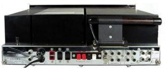
**BACK PANEL:** Scope outputs: TP 1 and TP 2. FUSE. Power cord. AC OUTLETS: 1 UNSWITCHED, 2 SWITCHED. Push terminals: GROUND, 300 OHM and 75 OHM ANTENNA. L+R OUTPUT. GrouND terminal. OUTPUTS: MAIN, TAPE. INPUTS: AUX, TAPE, PH 1, PH 2. Panloc mounting.
