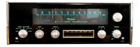
**FRONT PANEL:** Glass with illuminated teal/gold nomenclature. Illuminated dial. Electron ray TUNING indicator. STEREO light. Tuning control. **FINDUT SELECTOR:** AUX, TAPE, FM, PH 1, PH 2. Dual concentric BASS and TREBLE controls. Pushbutton switches: MONO or STEREO, LF: IN OF OUT, HF: IN OF OUT, TAPE monitor: IN OF OUT, MUTING: IN OF OUT, LOUDNESS: IN OF OUT. BALANCE. VOLUME with on-OFF switch. PANLOC buttons.
