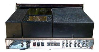
**BACK PANEL:** Scope outputs: TP 1 and TP 2. FUSE. Power cord. AC OUTLETS: 1 UNSWITCHED, 2 SWITCHED. FM ANTENNA SCREW terminals. L+R OUTPUT. Ground terminal. OUTPUTS: MAIN, TAPE. INPUTS: AUX, TAPE, PH 1, PH 2. Panloc mounting.
