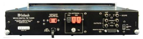
BACK PANEL: UNSWITCHED AC outlet. Power cord. Push terminals for: GND, 300  $\Omega$  FM ANTENNA. 75  $\Omega$  FM ANTENNA coax input. Scope outputs: VERTical (TP1) and HORIZONTAL (TP2). Audio OUTPUTS: Left & Right 2.5V VARIABLE and 1V FIXED. 15 pin REMOTE CONTROL receptacle. MANUAL AFL switch: OUT or NORMAL. Panloc mounting.
