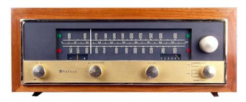
FRONT PANEL: Anodized gold and black aluminum panel. Illuminated dial. FM light. AM light. Tuning indicator: - to +. Signal strength indicator: 0 to 5. MC light. KC light. Tuning control. ← AFC control: MIN to MAX. AM SENSITIVITY switch: greatest, intermediate or minimum. VOLUME control with on-OFF switch. SELECTOR switch: FM LISTEN, FM TUNE, AM BROAD, AM MEDium, AM SHARP or PHONO.
