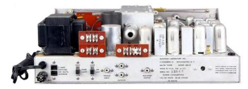
BACK PANEL: Screw terminals for to tv set, FM 300 Ω ANTenna, and AM ANTenna: HI, LO and GND.
