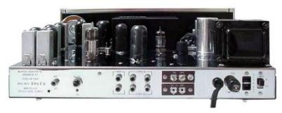
**BACK PANEL:** MPX OUTPUT. MUTING ADJUSTMENT. MONO OUT (2). STEREO IN. STEREO OUT. Screw terminals: FM ANTenna and TO TV SET. Power cord. FUSE. Unswitched AC outlet. LAMPS switch: High and Low.
