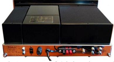
**BACK PANEL:** TP1 and TP2 scope outputs. Switched AC outlet. FUSE. Power cord. Push terminals for FM ANTenna: GND,  $300~\Omega$  FM ANTenna.  $75~\Omega$  FM ANTenna coax input. LEFT & RIGHT AUDIO OUTPUTS: 2.5V FIXED OUTPUT and FRONT PANEL CONTROLLED. Panloc mounting.
