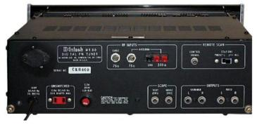
BACK PANEL: RFINPUTS: 75 Ω CABLE and ANTENNA coax inputs. Push terminals for GND and 300 Ω ANTENNA. REMOTE control SCAN: CONTROL SIGNAL jack. STATIONS switch: PRESET OF ALL.
